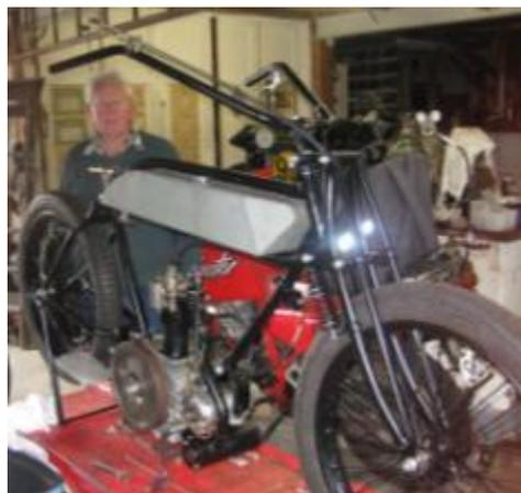
The first thing to do was to strip the engine unit which has an overhead inlet and side exhaust design. Incorporated is a two speed gearbox, the gears being of a cone clutch design, operated by a rocking pedal, all quite simple with the gearbox being in front of the engine which runs backwards. A couple of bearings were replaced so the shafts could be set up correctly. It all appears to work well, on the bench at least.
